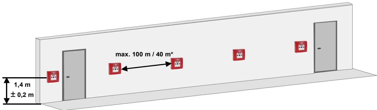
Fig. 30: Configuration of manual call points (MCP)
